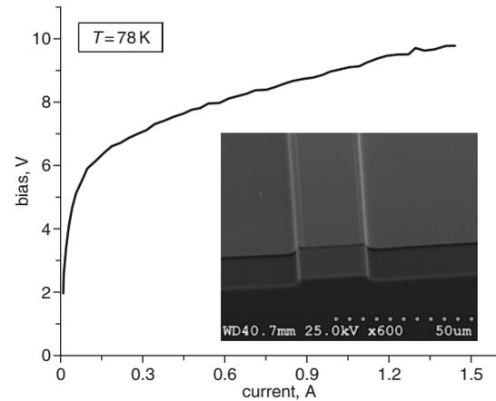
**Fig. 1** Current-voltage characteristic at 78 K of ridge laser device (width = 24  $\mu\text{m}$ , length = 1.5 mm) Differential resistance, when structure aligned,  $\approx 2.8 \Omega$  Inset: Scanning electron microscope image of cavity facet of typical device
