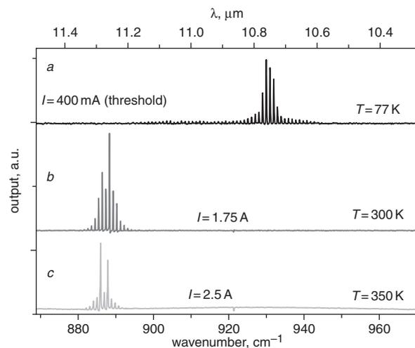
**Fig. 2** Spectra of selected devices at 77, 300, 350 K
