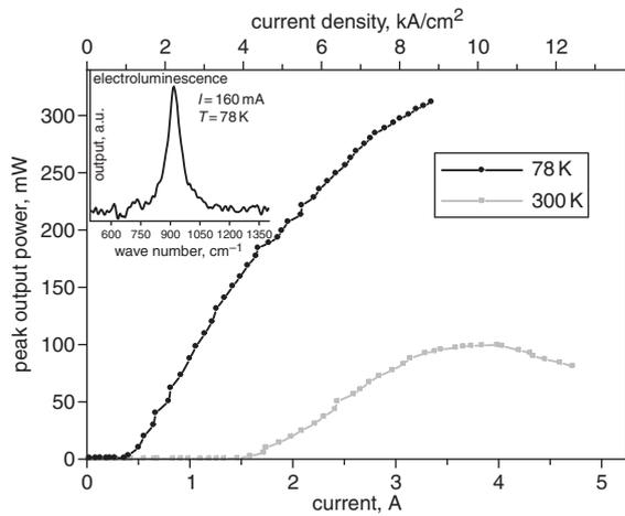
**Fig. 3** Light-current characteristic of typical device (ridge width = 24  $\mu\text{m}$ , cavity length = 1.5 mm) at 77 and 300 K
