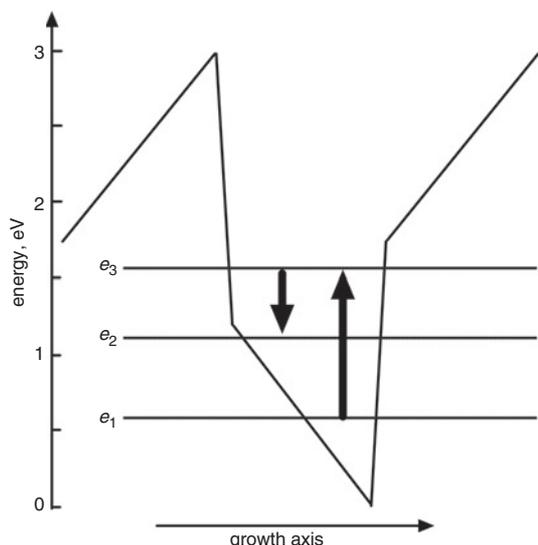
**Fig. 1** Conduction band profile and energy levels of GaN/AlN quantum wells
