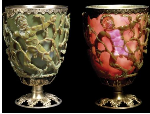
Figure 1.1: The Lycurgus glass cup, demonstrating the bright red color of transmitted light though gold nanocrystals [28].
